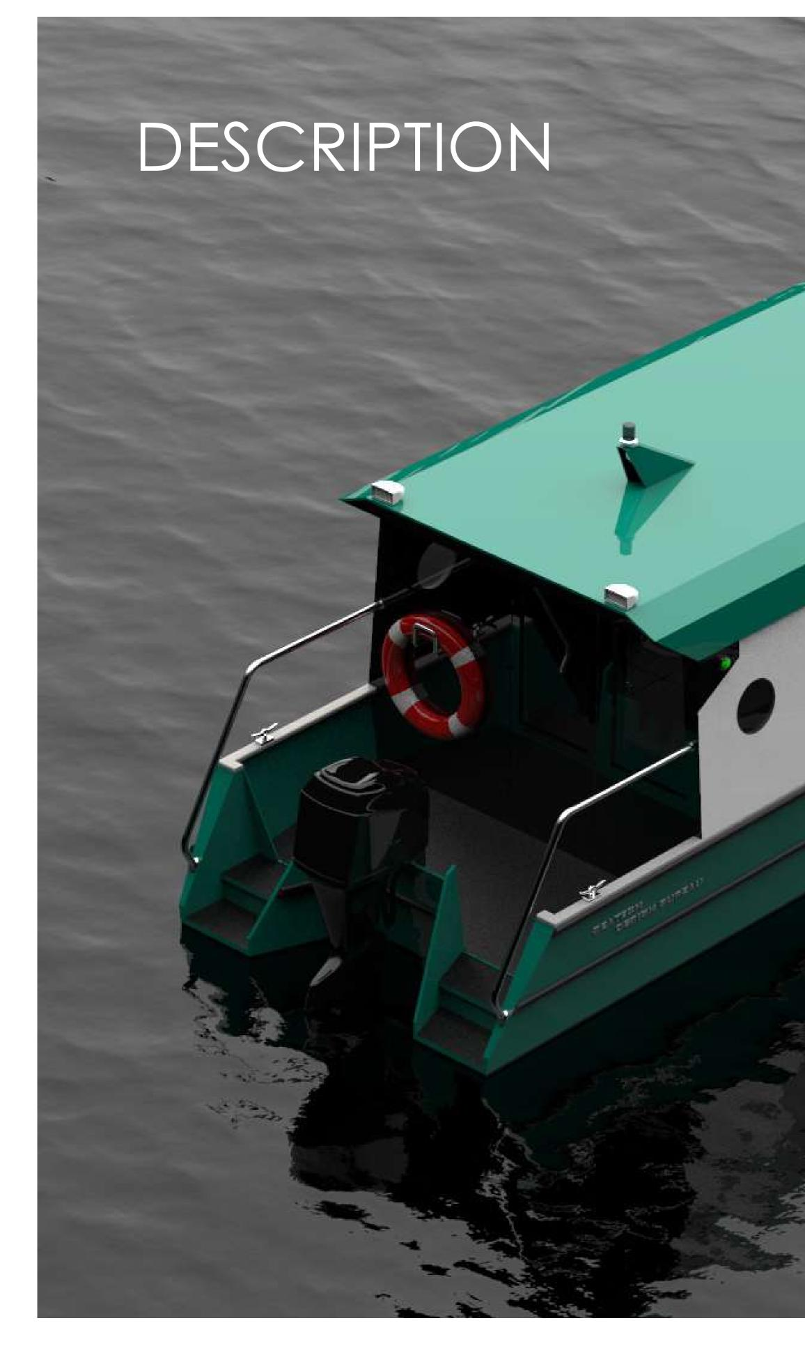
We present a "Raznezhie-6" model range of leisure boats based on combination of sets of module structural elements of hull and superstructure. Adding various elements to the base hull, which is a ready-to-use openboat, customer can get a number of boat models for different types of water recreation. Vessel can be used as from recreational fishing boat to cruise boat and minihouseboat.
